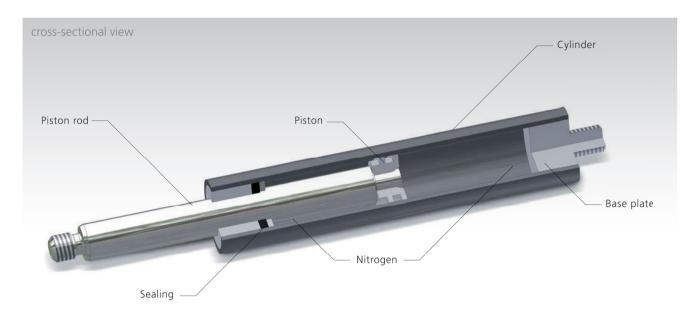
HAHN gas springs are hydropneumatic, closed and maintenance-free adjustable elements. The spring force F1 results from the internal pressure (160 bars without load at the most) in the cylinder, which is generated by the filling medium nitrogen.
