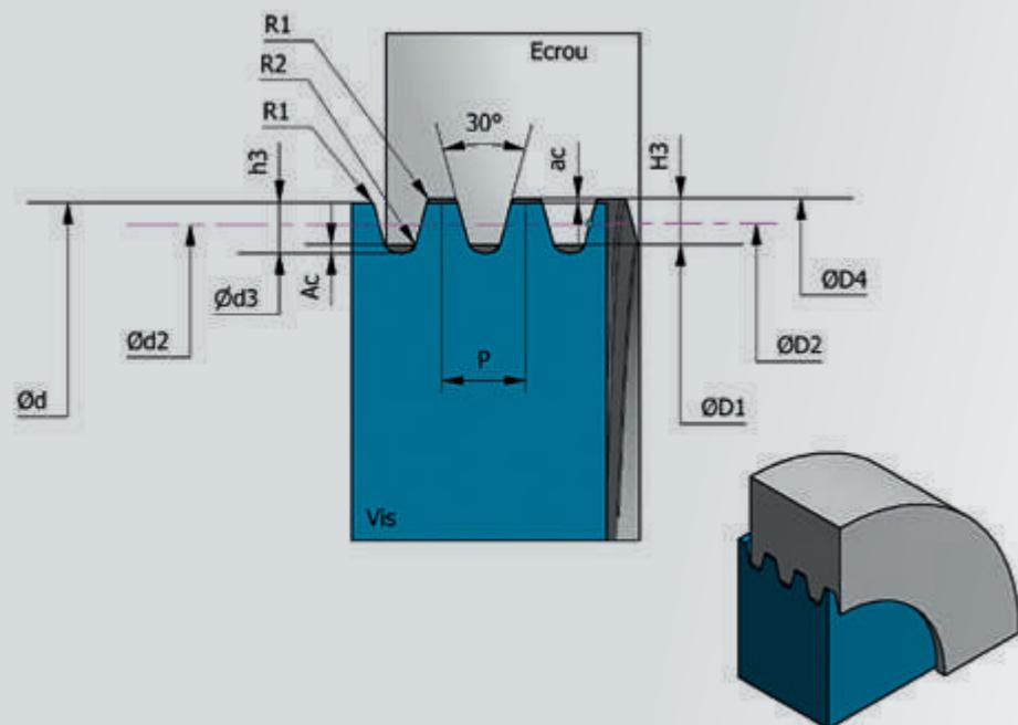
$\varnothing d$  = nominal diameter of the thread
