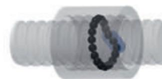
For nuts with several threads, the solution is a tubular duct in the periphery of the nut. The system enables the transfer of balls from one end of the nut to the other.
