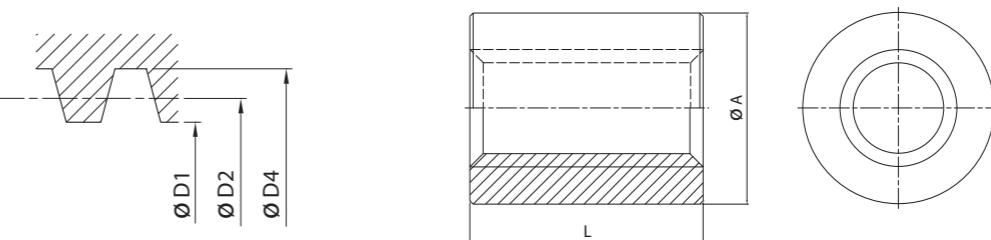
Material: 11SMnPb37 (1.0737) / 11SMn37 (1.0736) Trapezoidal in accordance with ISO 2901/2903 and DIN103, 7H tolerance
