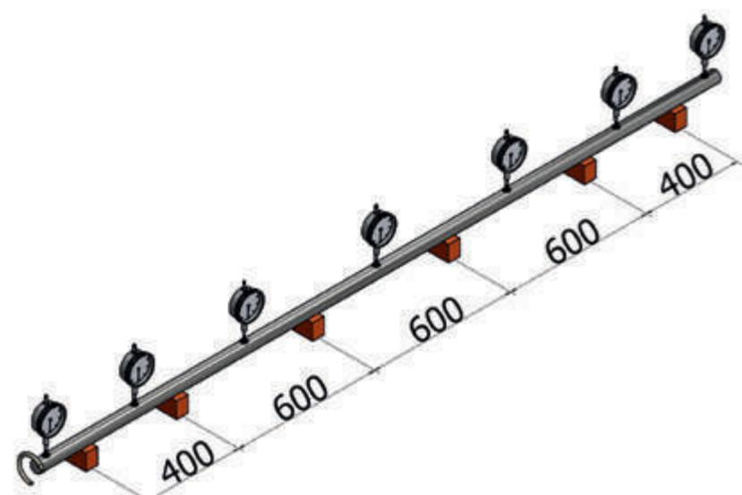
**Example:** for a given reference with a rectitude of 0.5, the value measured on each comparator, spaced as shown in the figure, must be less than 1mm for a full revolution of the bar.
