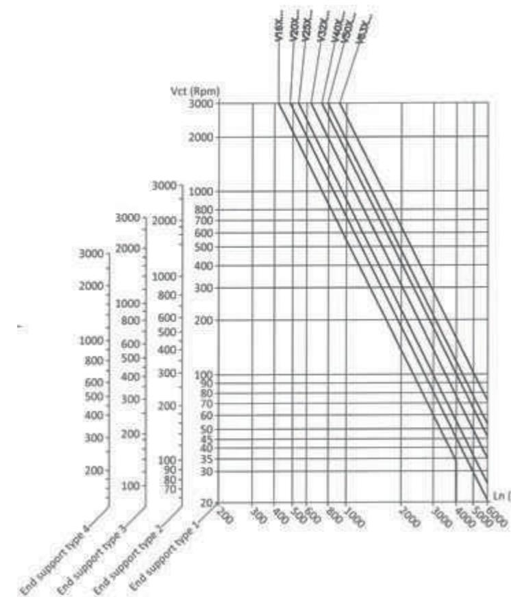
We recommend regular checks are performed to ensure that the acceptable maximum speed is compatible with the nut's recycling system:
