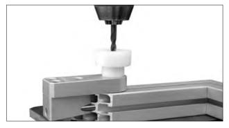
**Use of MiniTec drilling jigs** Slide jig in central bore of the mitred profile to the stopper. Tighten with screw. Insert ino profile with bore through the drilling guide inside the fixing screw.
