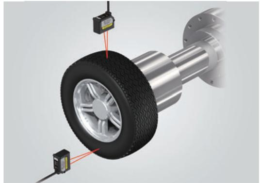
Dark surfaces absorb light, which used to make measurement difficult. But automatic brightness control now makes stable detection possible. The IL Series produces reliable run-out readings by observing run-out in multiple areas.
