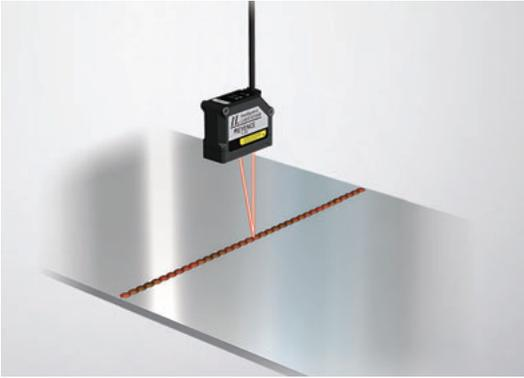
Conventionally, uneven surfaces from welding seams would alter the amount of reflected light, causing inconsistencies in appearance that would lead to unstable detection. The IL Series provides stable detection through its automatic brightness control function.
