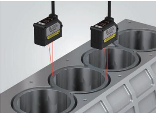
Conventional systems are easily influenced by the likes of stains and bumps on metal workpiece surfaces, but automatic brightness control enables stable detection. Measurement data can be processed for multiple points at once, making parallelism checks possible.
